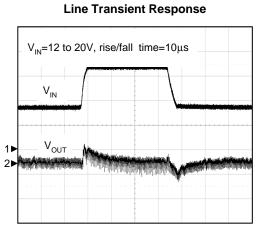
CH1: V<sub>IN</sub>, 5V/Div, DC CH2: V<sub>OUT</sub>, 50mV/Div, offset=3.3V TIME: 50 $\mu$ s/Div
