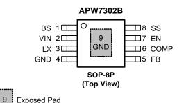
The pin 4 must be connected to the pin 9 (Exposed Pad)
