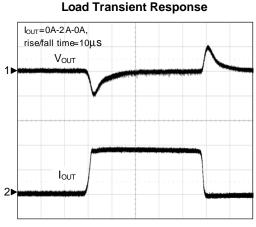
CH1: V<sub>OUT</sub>, 200mV/Div, offset=3.3V CH2: I<sub>L1</sub>, 1A/Div, DC TIME: 50 $\mu$ s/Div Load Transient Response
