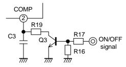
Fig.35 ON/OFF control circuit (2)
