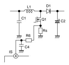
Fig.24 IS pin circuit
