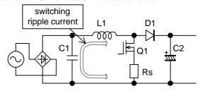
Fig.27 Input capacitor circuit
