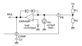
Fig.26 Input/output of error amplifier circuit
