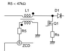
Fig.16 ZCD pin circuit
