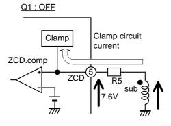
Fig.11 Clamp circuit of ZCD pin(2)
