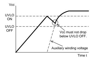
Fig.20 Vcc voltage at startup
