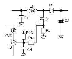
Fig.32 Compensation circuit of surge current
