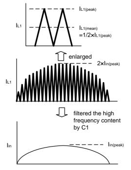
Fig.3 Outline of inductor and AC input current
