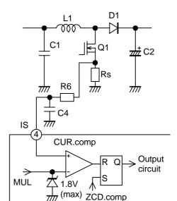
Fig.8 Current sense comparator circuit
