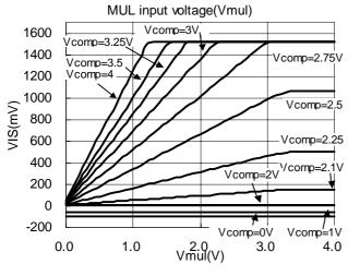
Current sense comparator thershold(VIS) vs. MUL input voltage(Vmul) (enlarged)
