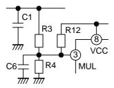
Fig.30 Compensation circuit of dead time
