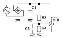
Fig.23 MUL pin circuit
