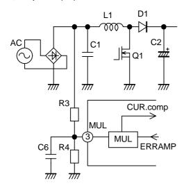
Fig.7 Multiplier circuit
