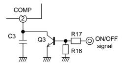
Fig.34 ON/OFF control circuit (1)
