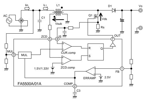
Fig.1 Outline of PFC converter circuit
