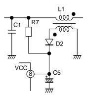
Fig.19 Vcc pin circuit
