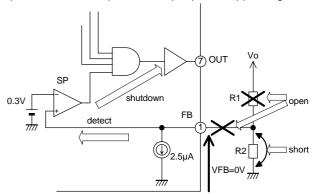
Fig.6 Open/short protection at FB pin
