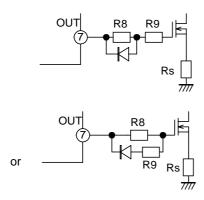
Fig.25 Gate drive circuit
