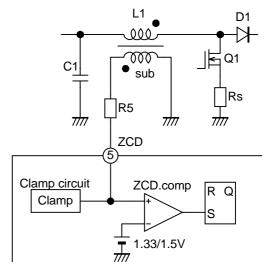
Fig.9 ZCD circuit
