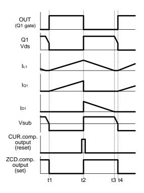
Fig.2 Timing chart of switching operation
