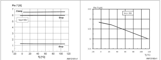
Figure 19. Latched disable threshold vs. junction temperature
