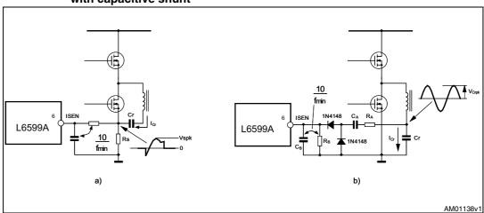
Figure 28. Current sensing techniques: a) with sense resistor, b) "lossless", with capacitive shunt
