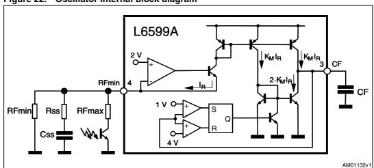
Figure 22. Oscillator internal block diagram
