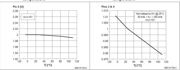
Figure 13. OCP delay source current vs. junction temperature
