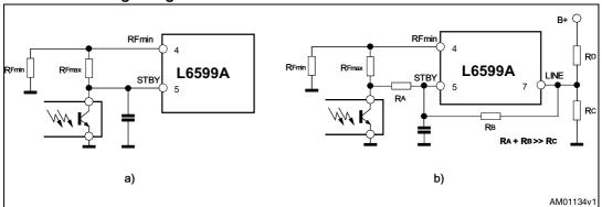
Essentially, RFmax defines the switching frequency fmax above which the L6599A enters burst mode operation. Once fmax is fixed, RFmax is found from the relationship:
