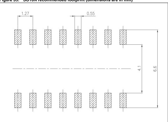
Figure 35. SO16N recommended footprint (dimensions are in mm)
