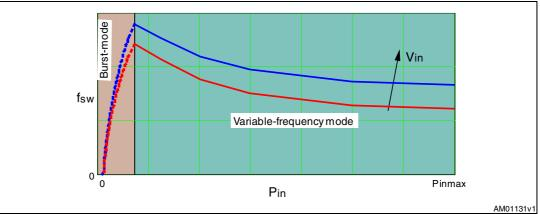
Figure 20. Multi-mode operation of the L6599A
