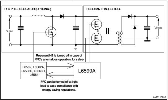
Figure 21. Typical system block diagram
