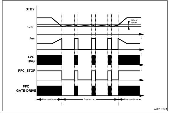
Figure 25. Load-dependent operating modes: timing diagram
