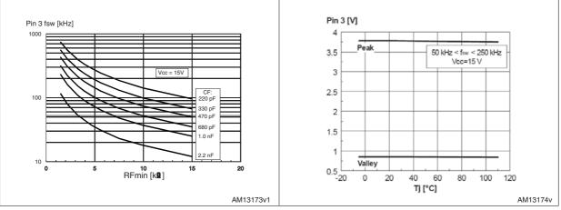
Figure 11. Reference voltage vs. junction temperature
