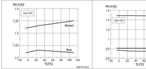
Figure 17. Line thresholds vs. junction temperature
