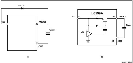
The diode prevents any current being able to flow from the VBOOT pin back to Vcc, in case the supply is quickly turned off when the internal capacitor of the pump is not fully discharged. To drive the synchronous DMOS a voltage higher than the supply voltage Vcc is necessary. This voltage is obtained by means of an internal charge pump (*Figure 31*b).
