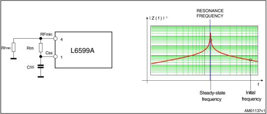
As a result, the average input current smoothly increases, without the peaking that occurs with linear frequency sweep, and the output voltage reaches the regulated value with almost no overshoot.
