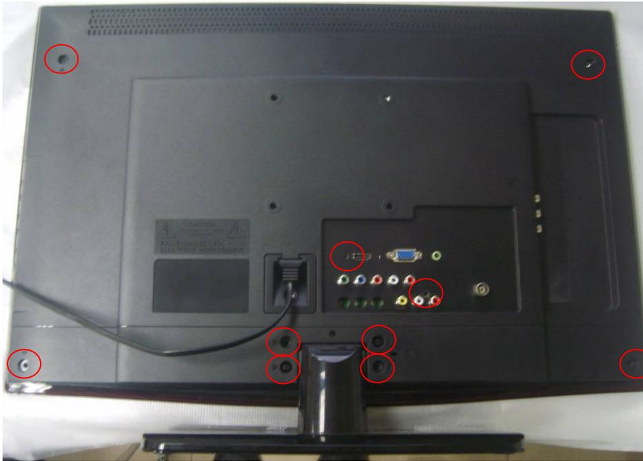
2. Remove the screws to remove AC cover.
