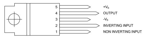
\*TAB CONNECTED TO PIN 3
